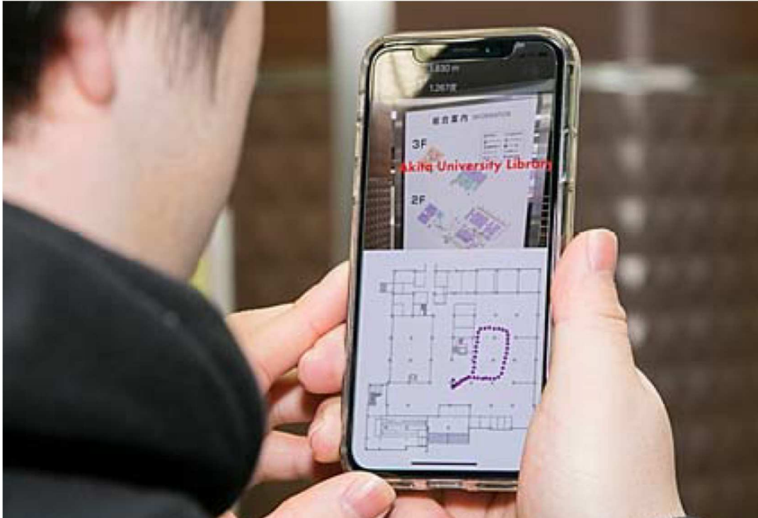
Figure 1. A prototype system of centimeter-level high-precision indoor navigation application on a smartphone using visual-inertial odometer
