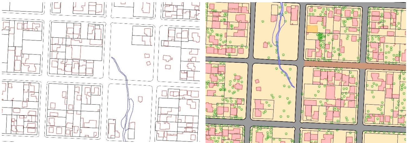
Figure 1. (a) Picture of a part of Cascavel topographic map with the old symbols and (b) with the newly proposed symbols.
