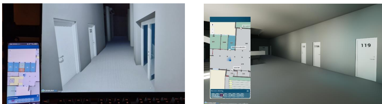
Figure 2a. The navigation application runs on a smartphone and is connected to the game engine running on a PC. Figure 2b. Screenshot of running simulation with an embedded navigation application.
