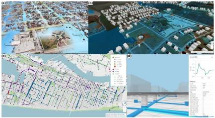
Figure 1. Street level and underground flood simulation for a flood event in Galveston
