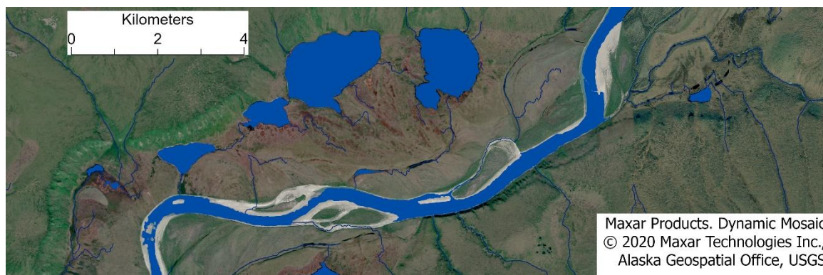
Figure 1. Sample of vector waterbodies and drainage lines (blue) in north-central Alaska predicted through deep learning and overlaid on high-resolution Maxar multispectral satellite image data.
