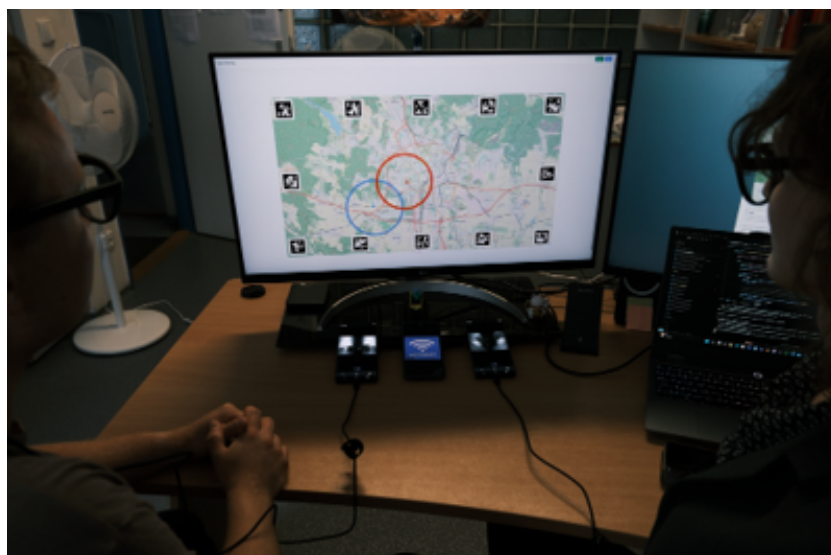
Figure 1. Proof-of-concept setup. Two participants wearing Pupil Neon eye-tracking glasses view a web map on a monitor. AprilTag markers around the screen perimeter provide spatial registration. Coloured circles appear as dwell-triggered pings, alerting the other participant to a point of interest.
