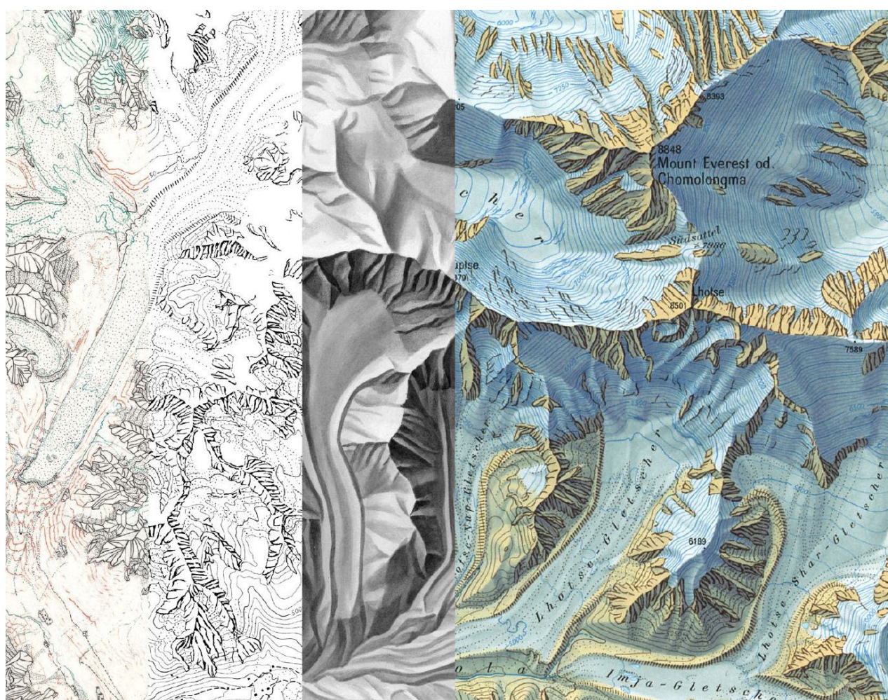
Figure 1. 1:100,000 colour relief map of Mount Everest in the Swiss Secondary School Atlas , 1962 edition. Eduard Imhof used the 1:25,000 Alpine Association map by Erwin Schneider from 1957 as a basis. From left to right: draft of the topographic line art elements, contour lines and rock areas; rock and relief originals; complete colour composite print of the map.
