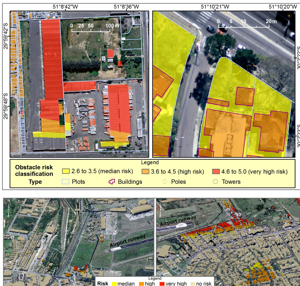
Figure 1. Parts of the obstacle risk classification map and 3D representation of the obstacles risk level.
