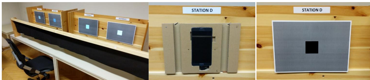
Figure 1. Lab setup for the study. Left: viewing stations with mobile phones of varying pixel densities mounted behind bezels, rail to ensure constant viewing distance, curtain to minimize reflections. Middle: mobile phone mounting fixture. Right: Bezel covering mounting fixture to reveal an area of identical size for each station.
