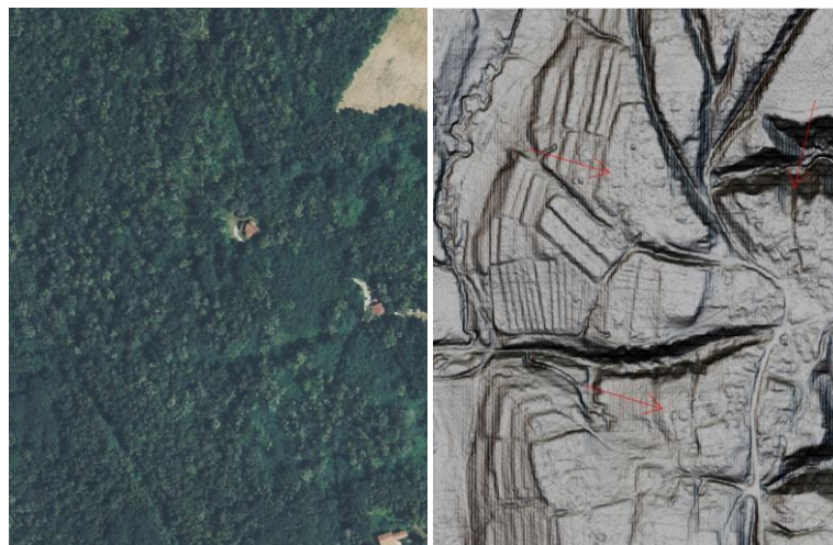
Figure 1. Unesco site of Castelseprio (Olona, VA) 3 . National cartographic geoportal, Color orthophoto 2006; On the right side: elaboration of the DTM as multiple Hillshade (D16-H10) on Slope visualisation
