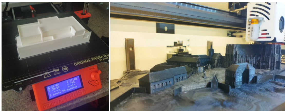
Figure 4. Small model of Villa Tugendhat with support structures manufactured using the Prusa i3 3D printer (left), large-size model manufactured using the Craftbot FLOW IDEX XL printer (right)
