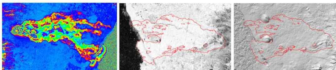
Figure 1: Interferogram (left), coherence (middle) and DTM (right)
