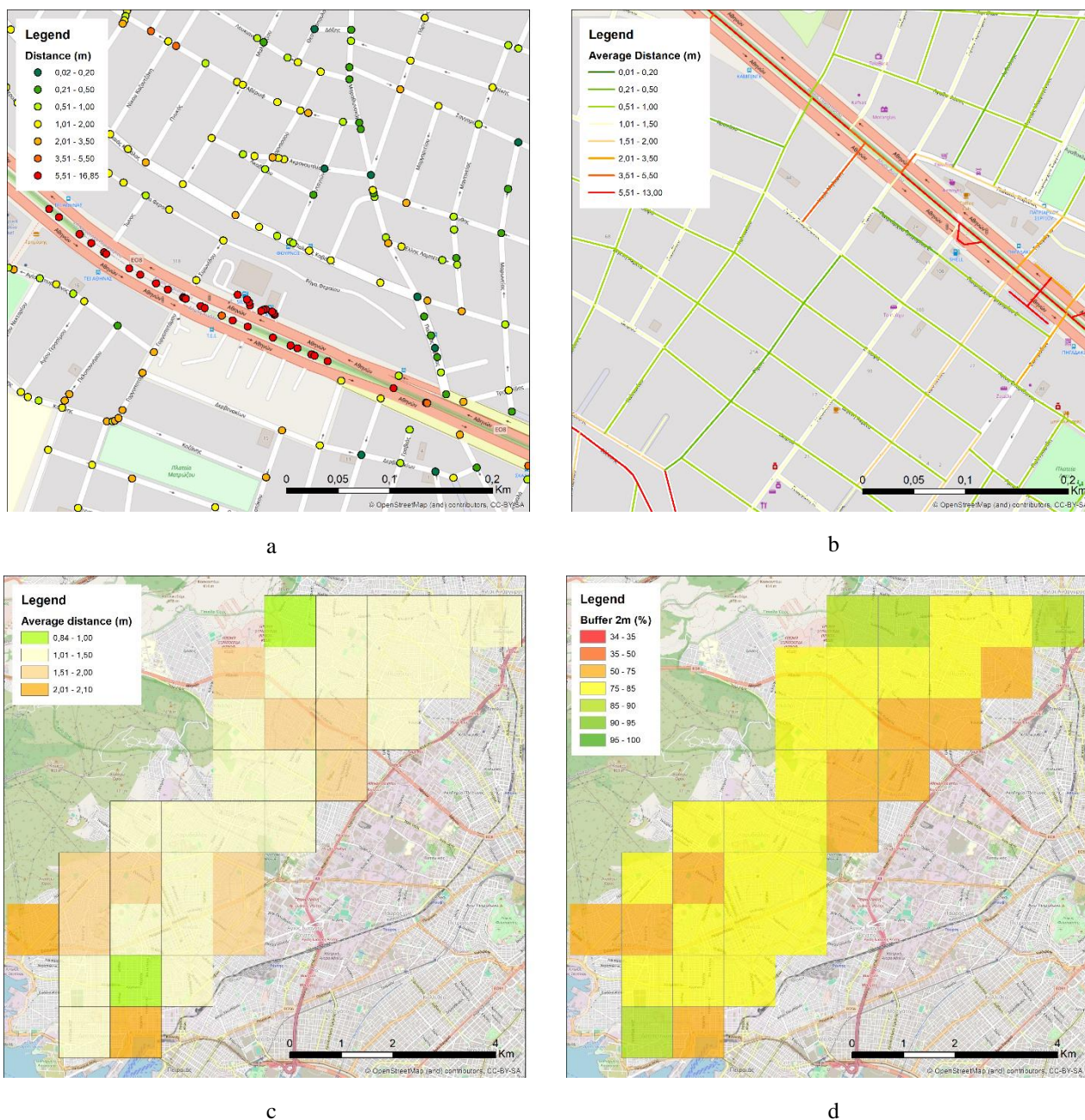
Figure 1. The positional accuracy of the road network can be evaluated and visualized at different levels of details Point/Vertex Level (1a), Line Level (1b) and Area / Grid Cell Level (1c) or (1d) to satisfy user needs.
