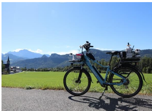
Figure 1. Instrumented bicycle equipped with LiDAR and a GNSS RTK receiver (source: Salzburg Research).
