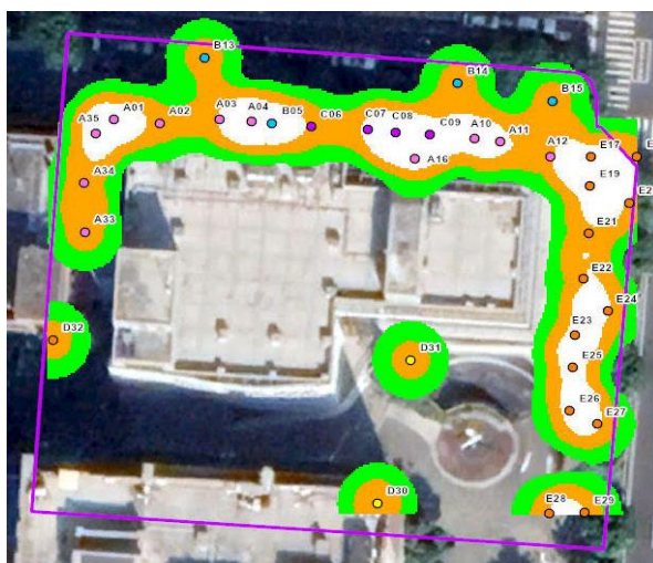
Figure 4. Example results of tree locations with a high area of influence (Rank 5 – white color), and low ranked value trees (orange and green color).
