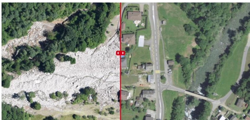
Figure 1 Example of the Rapid Mapping Service comparing pre- and post-disaster data based on a debris flow, Miso, June 2024. Left: post-disaster situation: Quick orthophoto 22.06.2024. Source: swisstopo/FOEN (2024). Right: pre-disaster situation: SWISSIMAGE, 2022. Source: swisstopo (2024).
